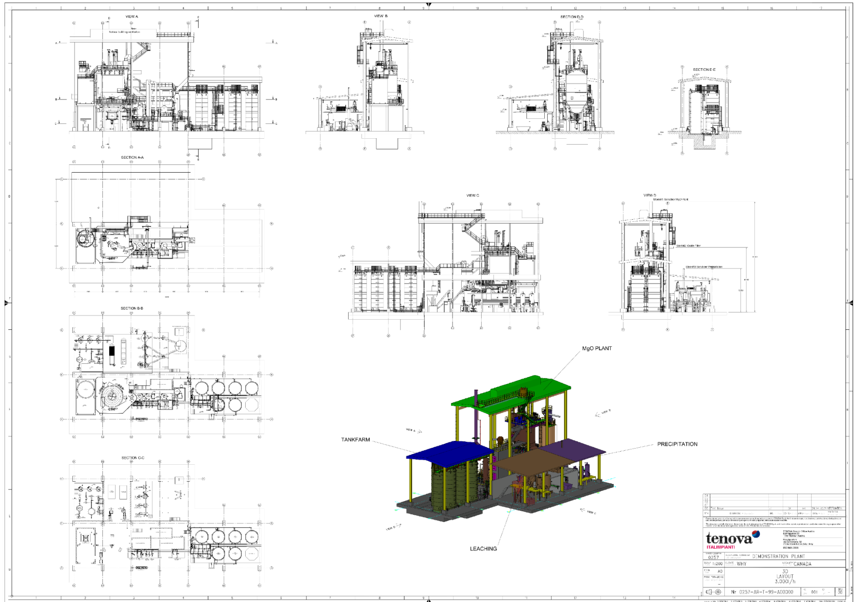
Figure 5: General Layout of Demonstration Plant – Equipment.
